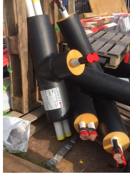
Image 34: Examples of the new PE-RT plastic pipes implemented in Østerby (Source: COWI)
